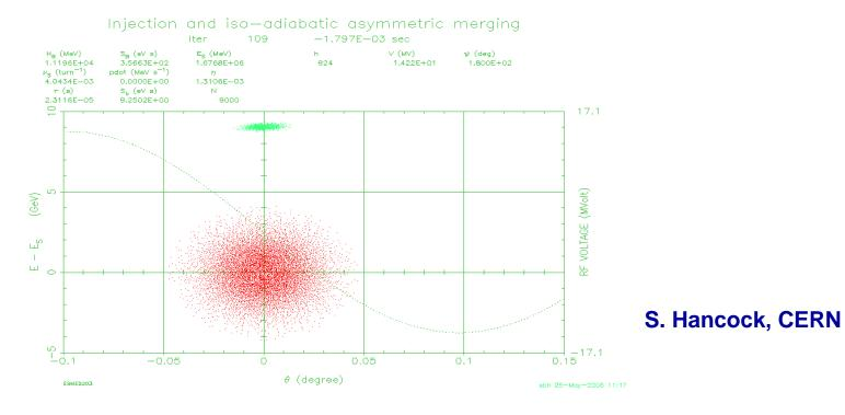
Stack and fresh bunch need to be positioned in adjacent "buckets" of the dual harmonic system (12.5 ns distance!)
