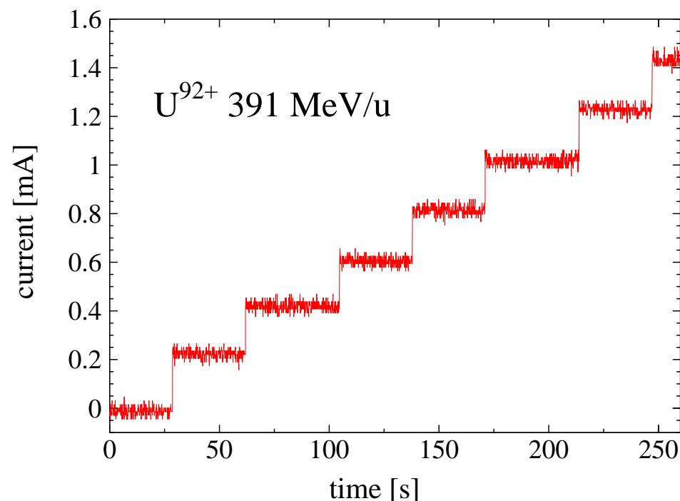
Accumulation rate limited by synchrotron cycle
