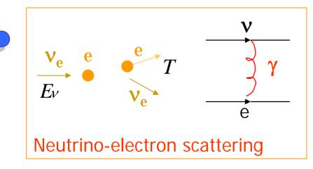
How can one measure  $\mu_v$ ? The presence of a magnetic moment introduces in the  $v_e$ -e cross section, a 1/T-like divergence, where T is the electron recoil energy.
