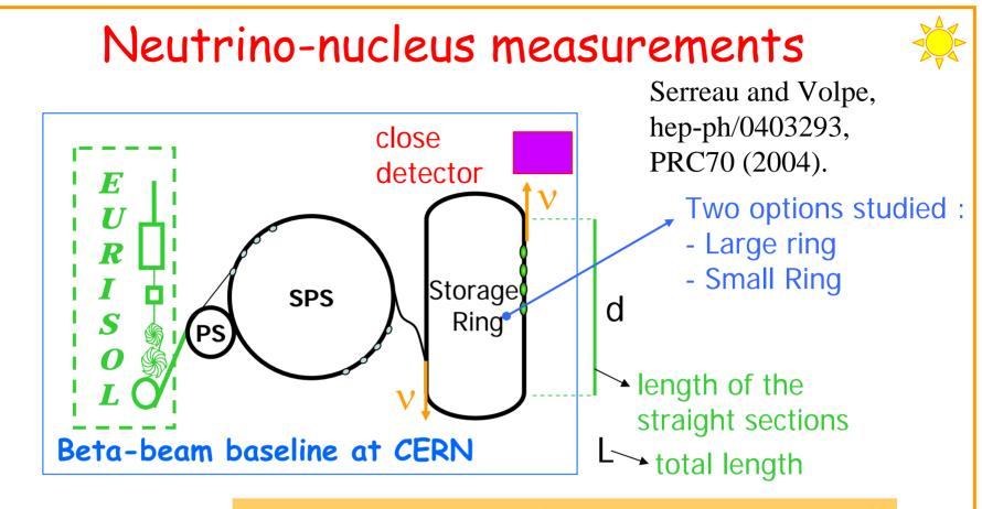
...or at one of the laboratories that will produce intense radioactive beams in the future (need of ion acceleration to GeV energy and of a storage ring).
