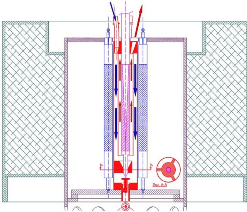
The inner geometry is characterized by three conical cavities having different angles and total length equal to the active height of the TRIGA core. The cone tip (lowest cone) is exposed to the highest power density for two reasons:
