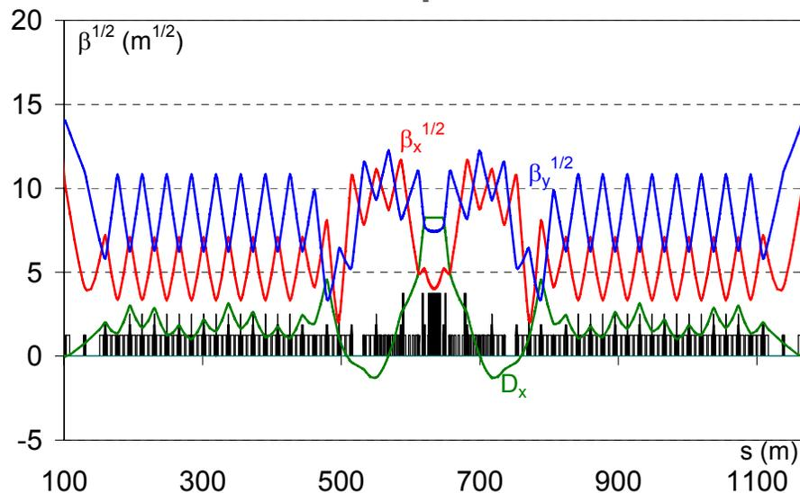
In the straight sections, we use FODO cells. The apertures are  $\pm 2$  cm in the both plans
