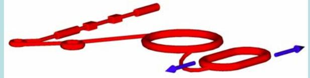
The  ${}^6\text{He}$  ions can be produced through a two step process. In the first stage protons hit a cooled robust primary target which can take a high beam power. The neutrons produced in the primary target will to large extent interact in the secondary target of Beryllium and produced  ${}^6\text{He}$  and  ${}^4\text{He}$ .
