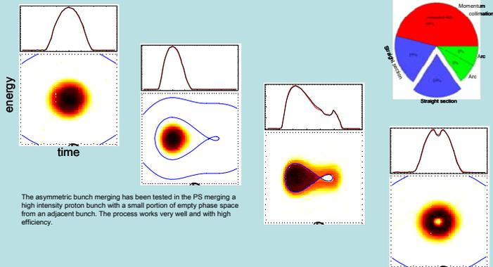
The asymmetric bunch merging has been tested in the PS merging a high intensity proton bunch with a small portion of empty phase space from an adjacent bunch. The process works very well and with high efficiency.
