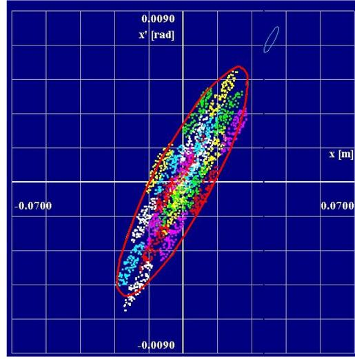
*Figure 5.4 Injected total emittance of  $80 \pi$ .mm.mrad after 41 turns with an incident beam emittance of  $1.5 \pi$ .mm.mrad.*
