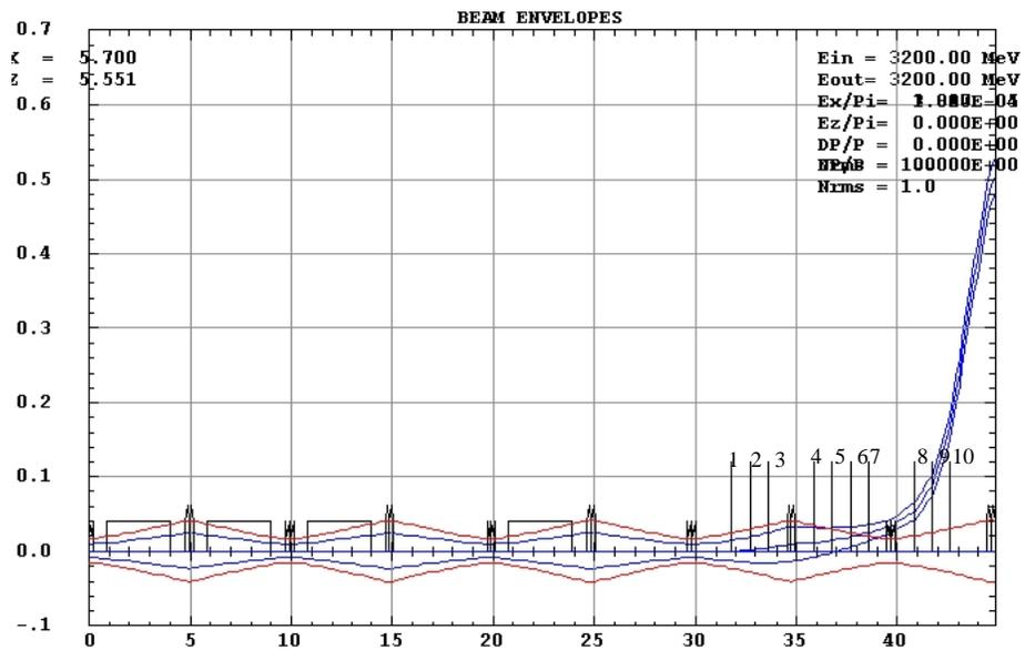
*Figure 6.1 Extracted beam ( blue line) and injected beam ( red line)*
