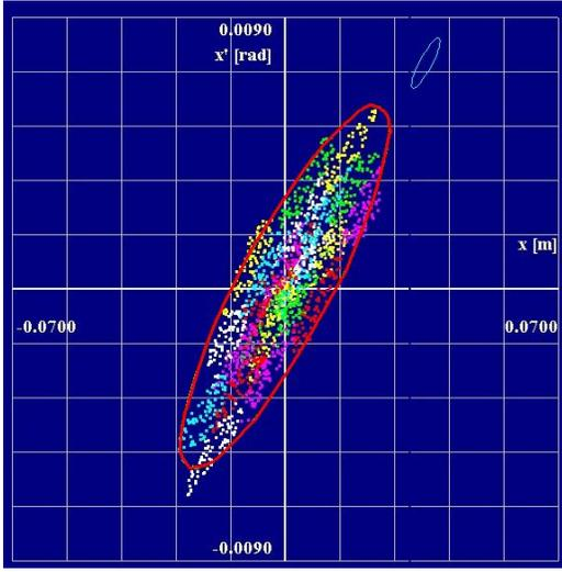
*Figure 5.3 Injected total emittance of  $80 \pi$ .mm.mrad after 41 turns with an incident beam emittance of  $1 \pi$ .mm.mrad.*
