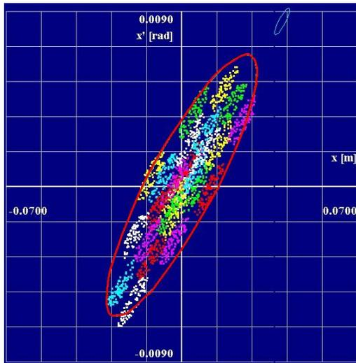
*Figure 5.1 Injected total emittance of  $100 \pi \text{ mm.mrad}$  after 41 turns with an incident beam emittance of  $1 \pi \text{ mm.mrad}$ .*
