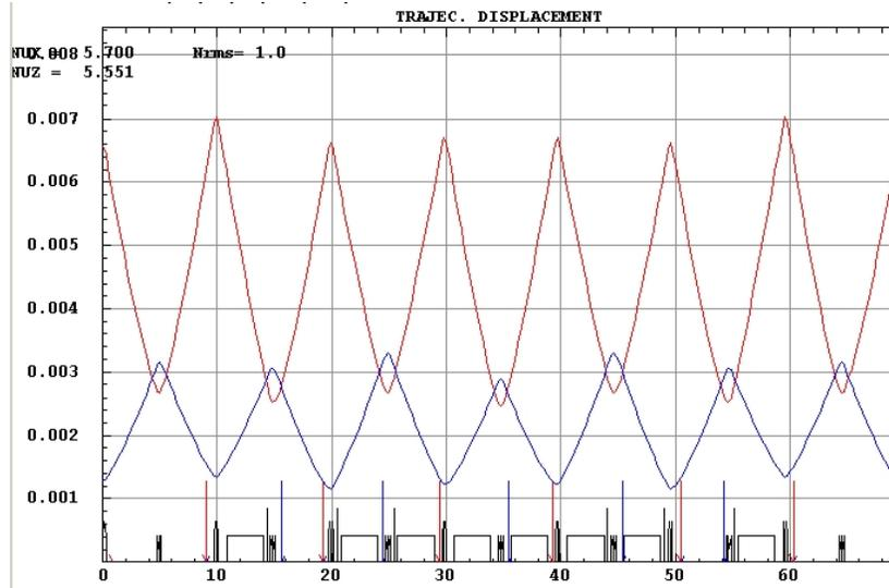
*Figure 4.3 RMS closed orbit distortion before correction*
