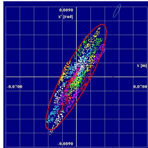
*Figure 5.2 Injected total emittance of  $100 \pi \text{ mm.mrad}$  after 41 turns with an incident beam emittance of  $1.5 \pi \text{ mm.mrad}$ .*
