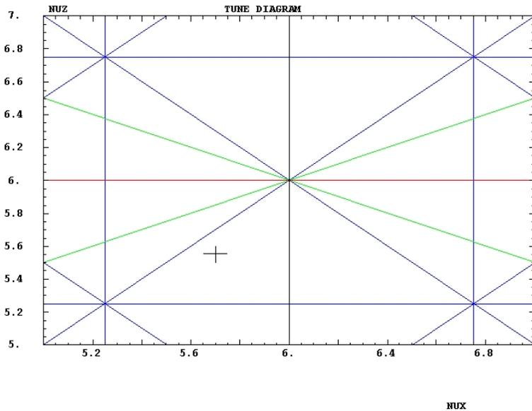
*Figure 2.2 Working point in the tune diagram with resonance lines up to the fourth order*
