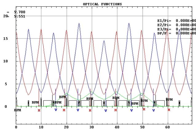
*Figure 4.1 Corrector and BPM location in the machine*
