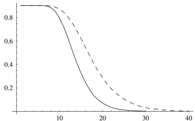
Figure 3: Survival profile of a single injected bunch versus number of stacking steps for helium (solid line) and neon (dashed line).
