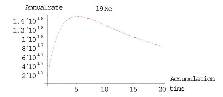
The annual neutrino rate as a function of the accumulation time in the EC-RCS and stacked in **PS** at 10 Hz injection.
