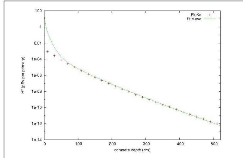
The MC calculations can be parametrized using an exponential function of the form:
