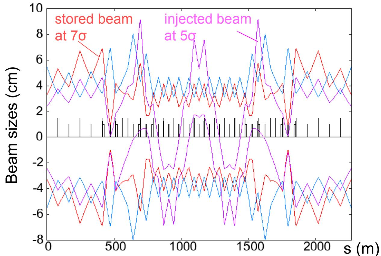
Large apertures needed for the dipoles and the quadrupoles
