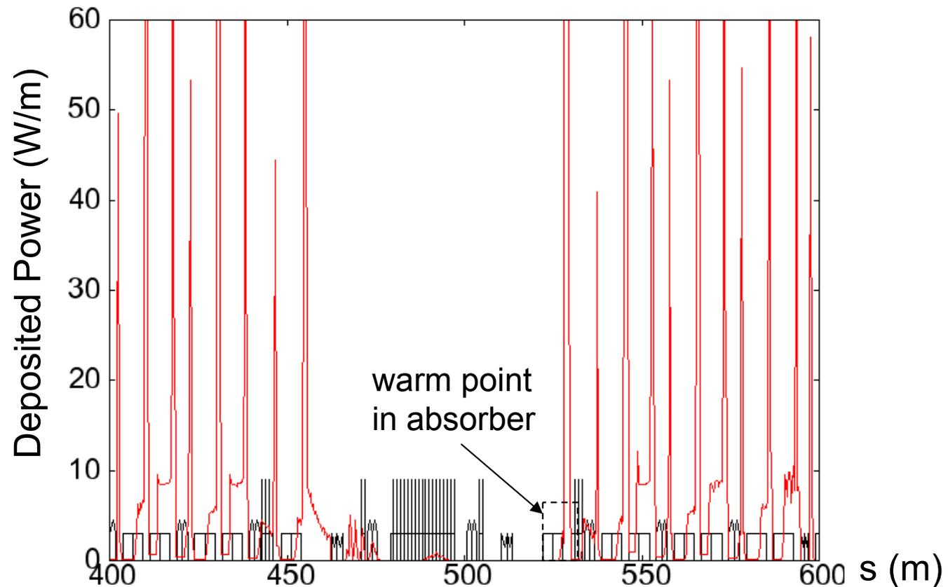
The absorber following the first dipole after the septum is a warm point. Several hundred of watts hit it continuously.
