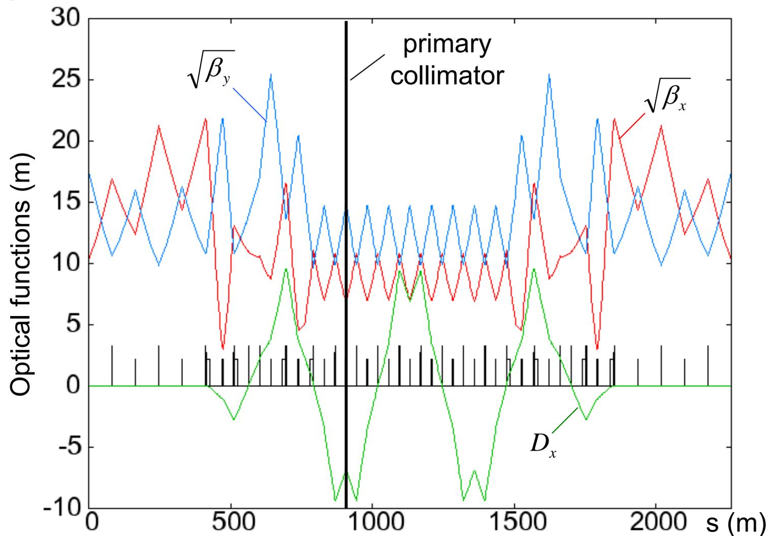
At the primary collimator, the normalized dispersion must be as high as possible. We have reached the value  $\frac{D}{\sqrt{\beta_x}} = 1 \text{ m}^{1/2}$  by doing a dispersion bump in the straight section.
