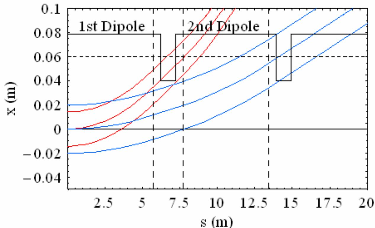
For  $^{18}\text{Ne}^{10+}$ , we need half-apertures of 8 cm in the dipoles to avoid the deposition of the decay products.
