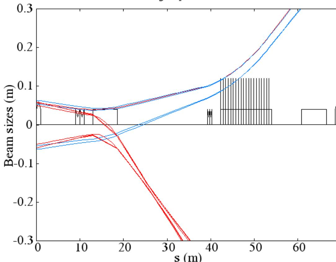
The beam sizes are at  $7 \sigma$  In red: Helium, in blue Neon
