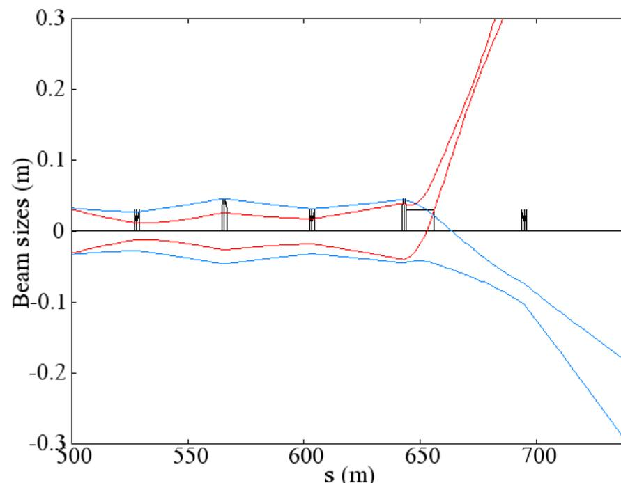
Left, beam of  $\text{Li}^{3+}(\text{F}^{9+})$  between the arc and the first dipole of the chicane
