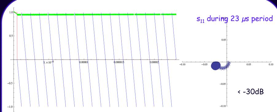
Blue: phase of drive current in units of  $\boldsymbol{\pi}$  (corresponding to frequency offset)
