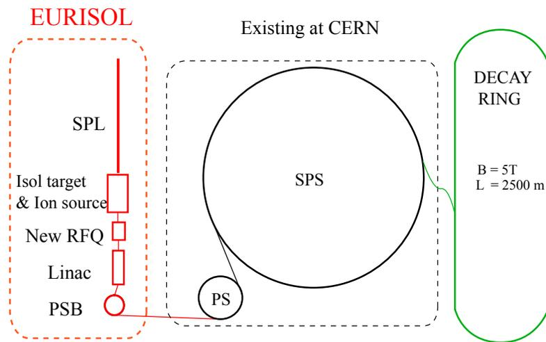
**FIGURE 1.** Schematic layout of the beta-beam complex. At left, the low energy part is largely similar to the EURISOL project. The central part (PS and SPS) uses existing facilities. At right, the decay ring has to be built.
