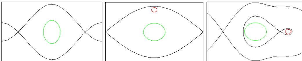
Figure 2: Bunch rotation stacking, longitudinal phase space plots (Energy versus Time):
