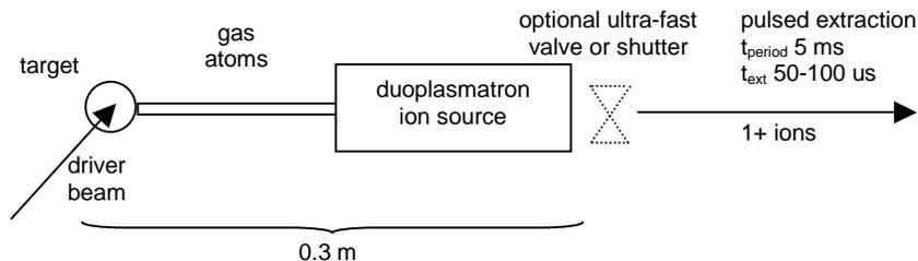
Fig. 4. Schematic layout of the gas injection into the duoplasmatron source.
