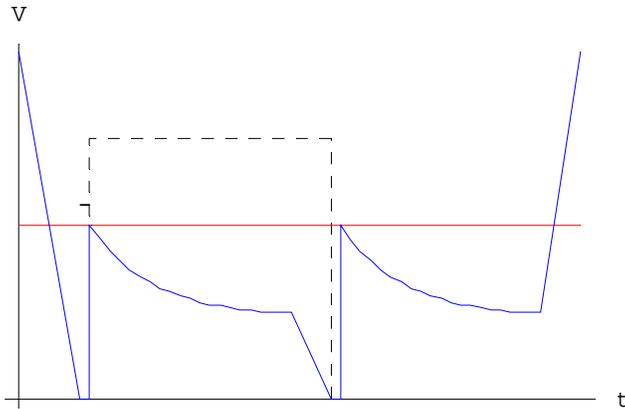
Figure 4: 40 (red) and 80 MHz (blue) voltage components during a single filling cycle. The dashed line indicates the portion repeated in the simulation.
