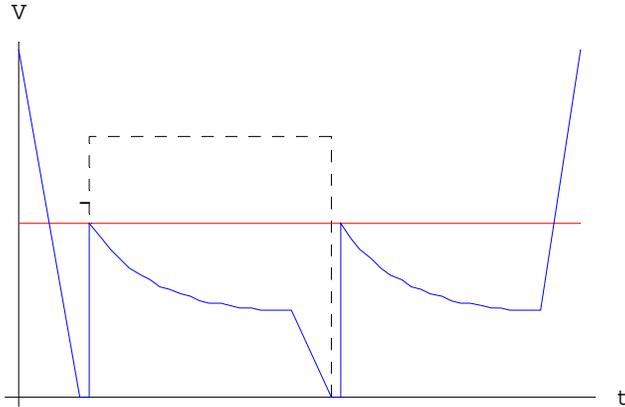
Figure 4: 40 (red) and 80 MHz (blue) voltage components during a single filling cycle. The dashed line indicates the portion repeated in the simulation.
